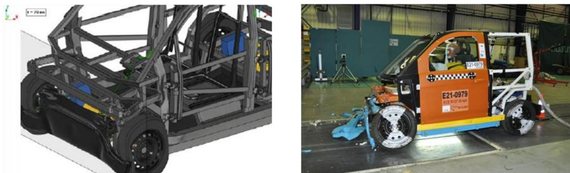
Fig. 5. Left: Vehicle status after frontal crash simulation. Right: General aspect of the vehicle after the frontal crash
