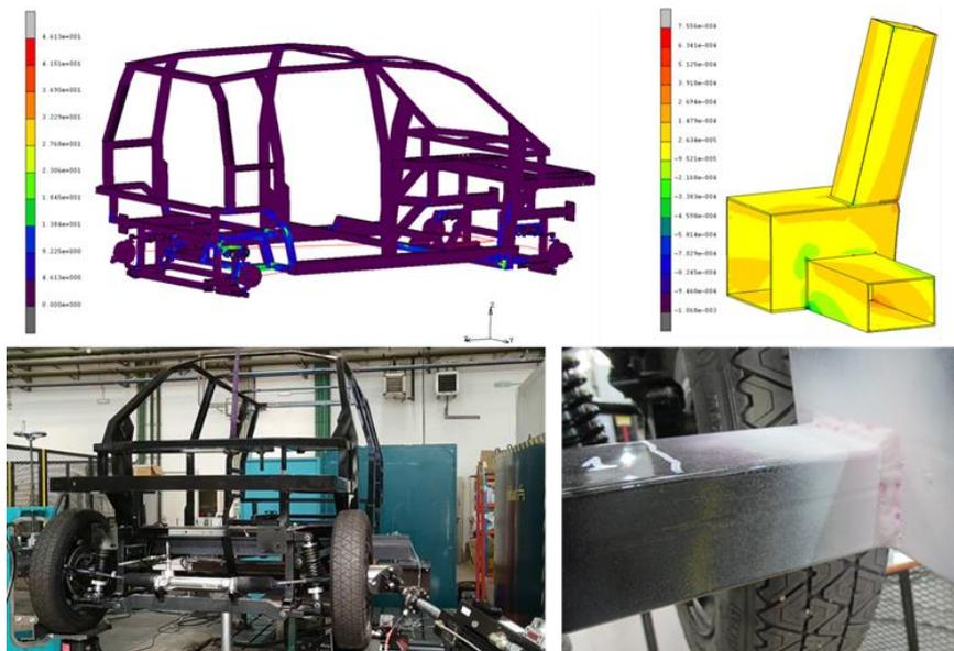
Fig. 4. Fatigue test results. Top left: equivalent von Mises stress results (MPa) during fatigue test simulation. Top right: strain distribution on a critical node. Bottom left: front part of the vehicle during fatigue experiments. Bottom right: penetrant liquids test on a critical node.
