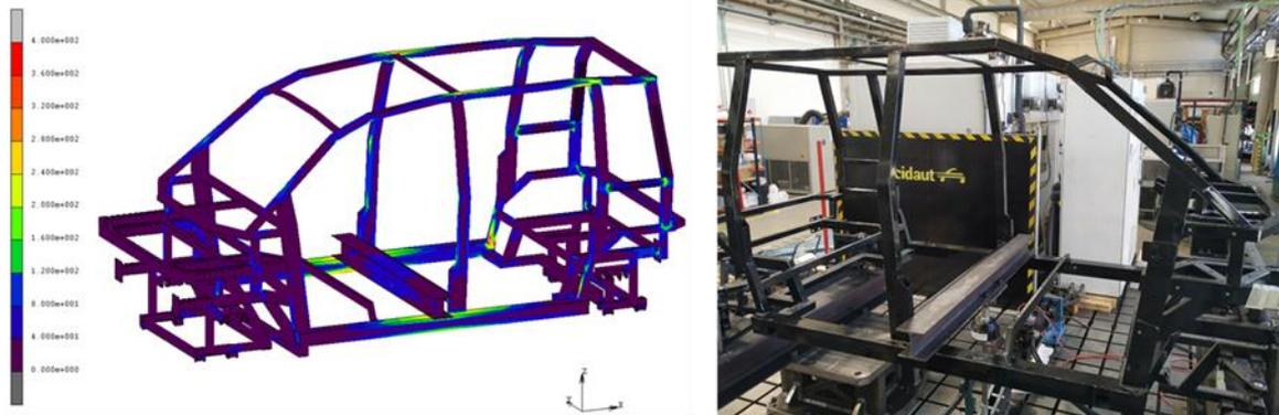
Fig. 2. Left: Equivalent von Mises stress (MPa) after bending test simulation. Right: Front part of the vehicle chassis during bending test.
