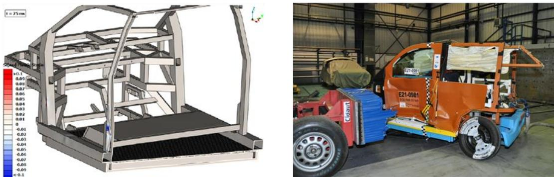
Fig. 7. Left: Plastic strain results after lateral crash simulation. Right: Overview of the vehicle after the lateral crash.
