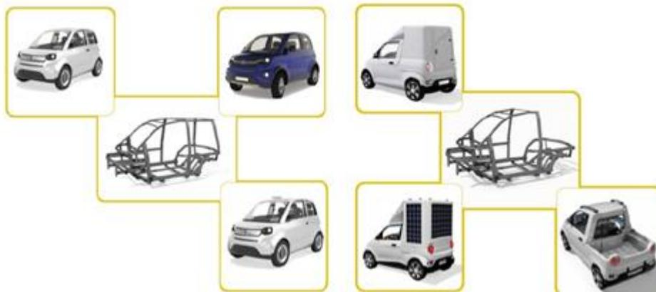
Fig. 1. Modular vehicle concept: very different vehicle architectures can be manufactured with minimal changes in the vehicle structure
