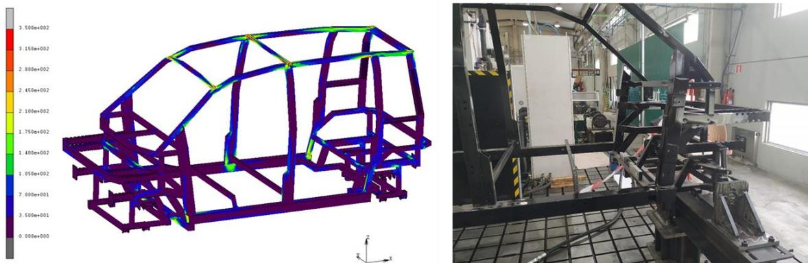
Fig. 3. Left: Equivalent von Mises stress (MPa) after torsion test simulation. Right: Front part of the vehicle chassis during torsion test.
