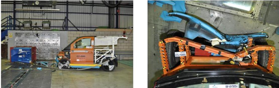
Fig. 6. Left: General aspect of the vehicle after the second frontal crash. Right: Deformation suffered by the structure after the second frontal crash.
