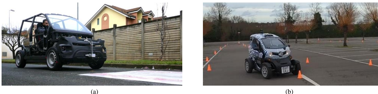
Fig. 1. (a) TELL/Multi-Moby EV prototype during a traction control test with a step change from high (dry tarmac) to low (white boards covered with water and soap) tire-road friction coefficient; and (b) ZEBRA EV during a U-turn test (passive configuration) in the car park of the University of Surrey, UK.
