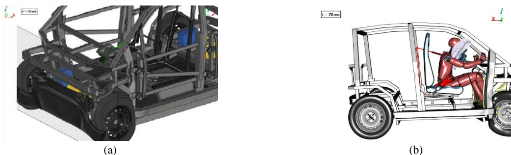
Fig. 2. (a) Simulation results of the Multi-Moby vehicle under the Regulation 137 (R137) crash, after structure optimisation; and (b) analysis of the restraint system under the R137 crash.
