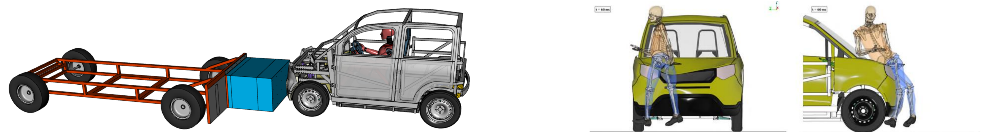
Figure 2. (Left) Frontal crash simulation. (Right) Pedestrian simulation with human model
